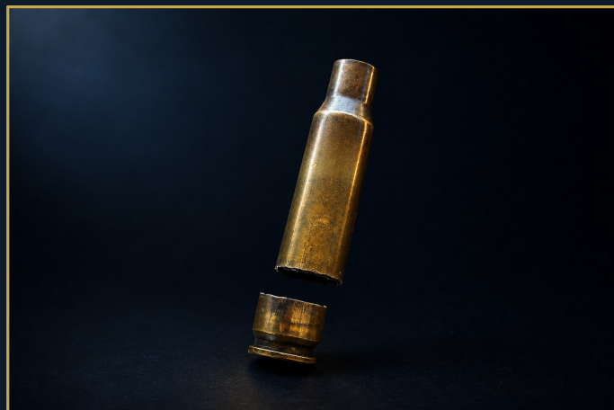
Case-head separation: the head has torn clean away from the body. This is what excessive headspace does when it's left to run.
