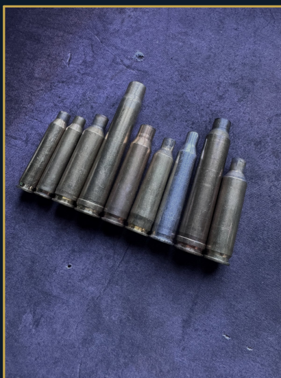
A working shooter's brass drawer. Every one of these headspaces on a different feature depending on its family.
