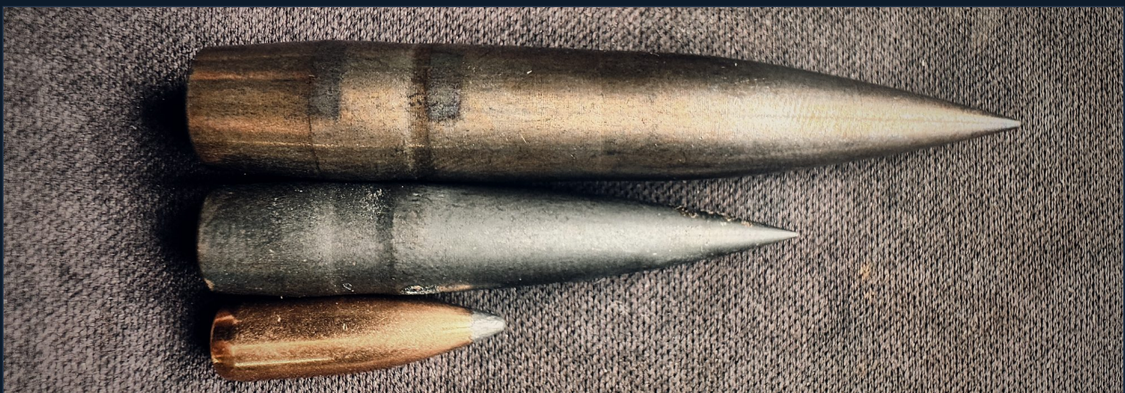
Three projectiles, three jobs: .375 CheyTac, .300 Win Mag, .223. The longer and heavier the bullet, the slower it leaves and the faster the twist it needs. Slow on purpose is a different job, not a quiet one.
